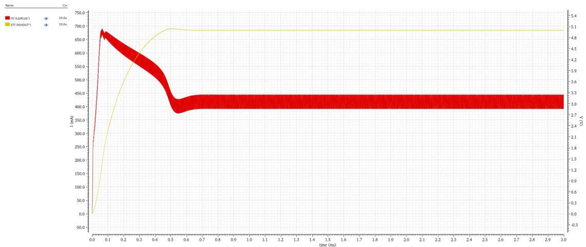
Figure 69: Results of starting up the converter with a 200 mA load
