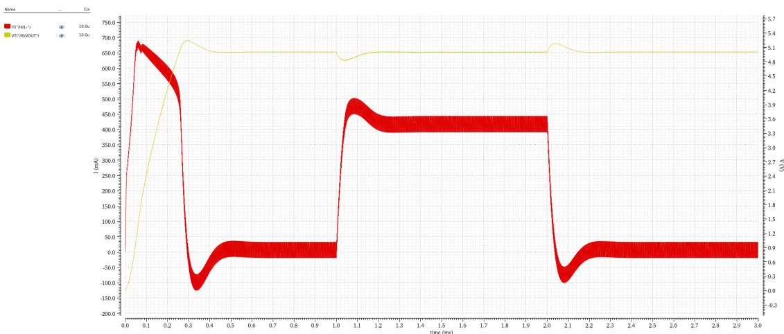
Figure 71: Results of applying a load step of 1 mA → 200 mA → 1 mA
